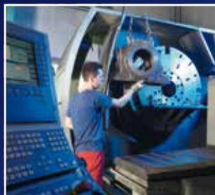
Expertise in manufacturing large bearing housings: components weighing over 4 t are machined with the greatest precision.
