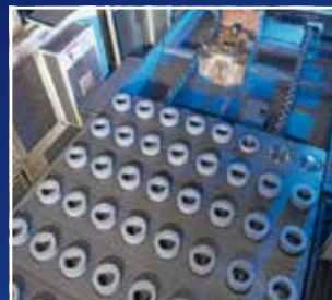
Quality production "round the clock": high-performance robots load the CNC turning centre with large-scale series parts.
