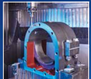
Latest modern manufacturing on a 5-axis machining centre
