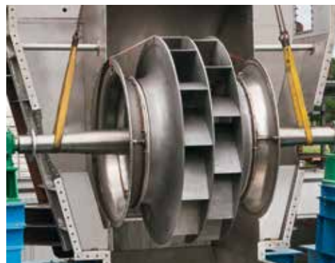
Example of application of HFB housings in modern, highly-loaded industrial fans
