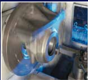
Machining a housing on a CNC turning centre
